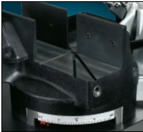
Easy-to-read frontal graduated scale. Escala graduada frontal de fácil lectura.
